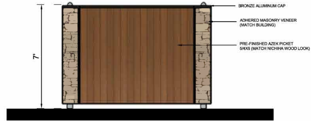
DUMPSTER ENCLOSURE - SIDE SCALE: 1/4" = 1'-0"
