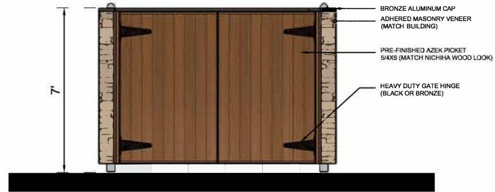
DUMPSTER ENCLOSURE - FRONT SCALE: 1/4" = 1'-0"
