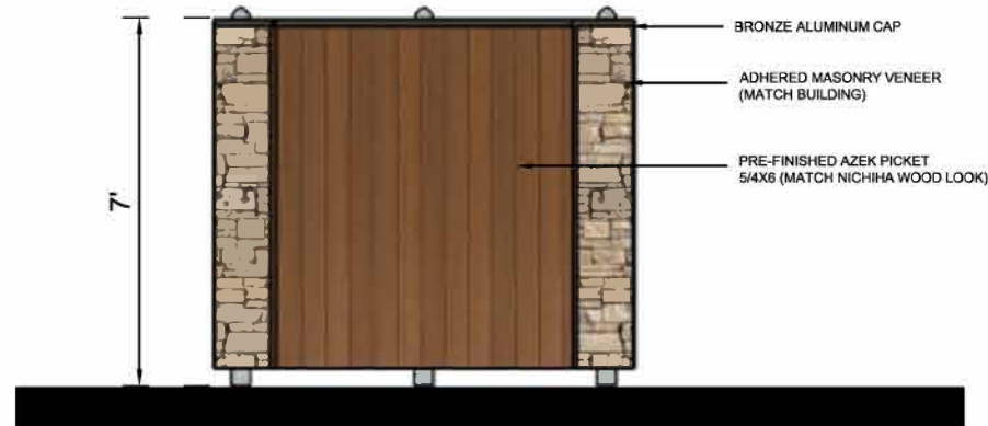
DUMPSTER ENCLOSURE - REAR SCALE: 1/4" = 1'-0"
